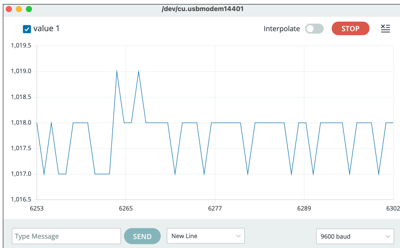
Figure A8.1b: Using the serial plotter turn the pot from one extreme to the other
