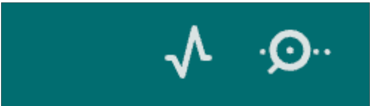
Figure 2: The serial plotter on the left and the serial monitor on the right
