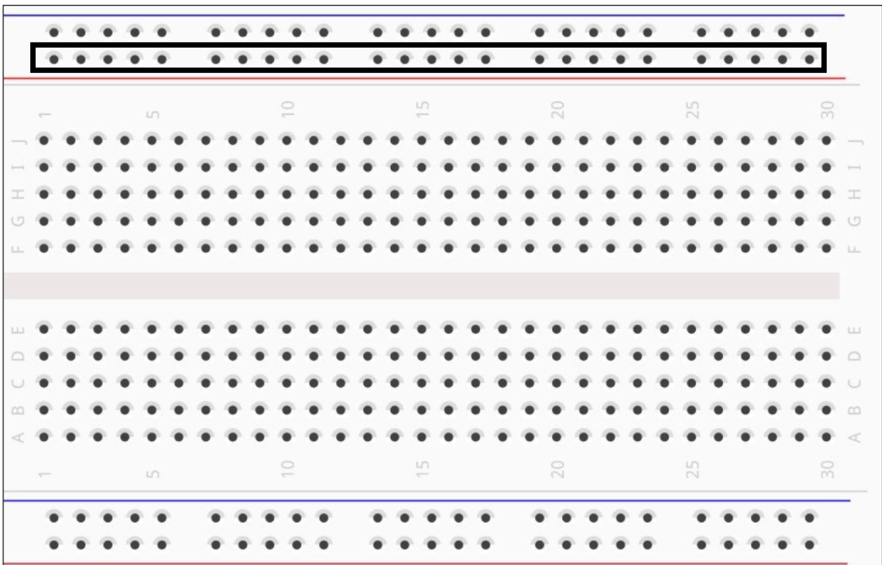
Figure 9: connecting along the length of the positive rail
